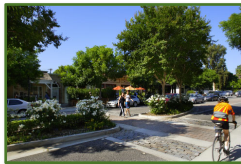
Figure 9-2 This example shows a pedestrian crosswalk with decorative paving, to help differentiate it from the road.
